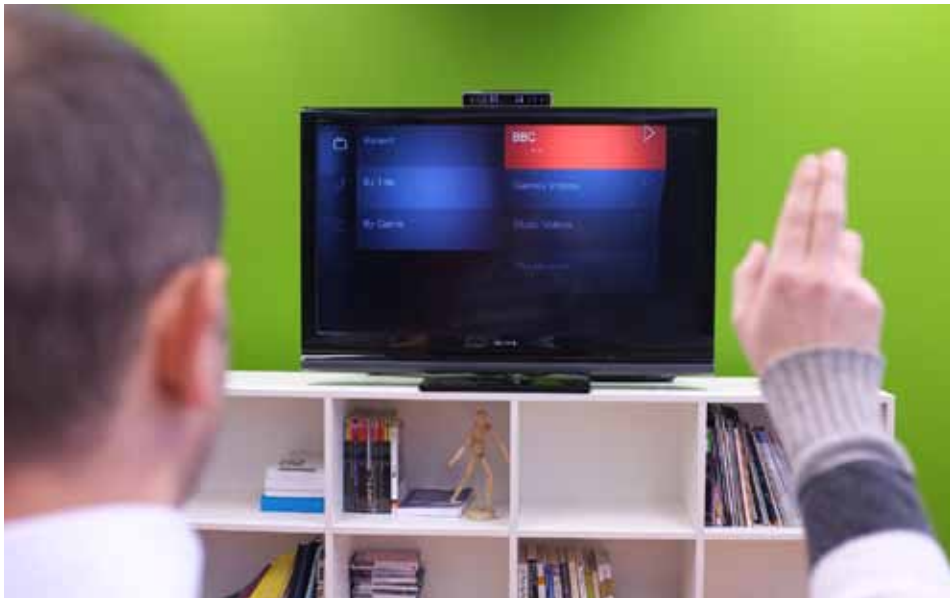
tracking The DepthSense camera can track the full body skeleton of several users up to four metres and individual fingers up to one metre.
