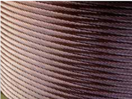
recycling Ecocopper is recycled by melting the scrap, refining it, and directly casting it into copper wire rod. (photos by Giovanni Dall'Orto)
